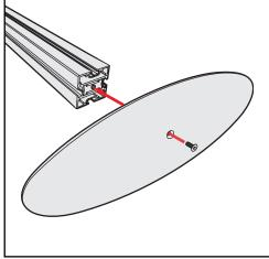
**Base Plate & Extrusion Connection**
